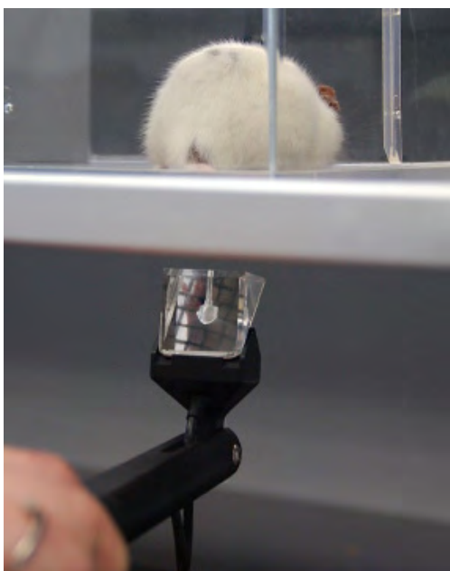
Fig. 1: "touch stimulator" with prism. Optional grid mesh not included
